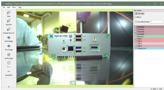
Figure 2. Objects of interest were labeled to generate a representative dataset of images for each type of PC, including components and missing or defective parts.
